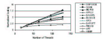
Fig. 4. Scaling of Amdahl's Speedup of OMPM2001 through 128 threads, normalized by the 16-thread speedup.
