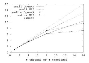
Fig. 2. Speedup of SPECseis for different data sets and programming models on a Sun Fire 6800 platform.
