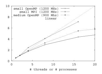
Fig. 3. Speedup of SPECchem for different data sets and programming models on a Sun Fire 6800 platform normalized by the 2-way speedup.
