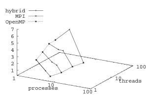
Fig. 11. Speedup of SPECchem for MPI, OpenMP and hybrid execution on a Sun Fire 15K. The lines connecting hybrid runs denote runs with the same number of processors\*threads.
