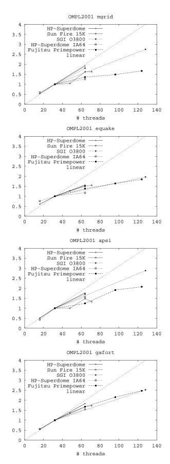
Fig. 7. Scalability of the OMPL benchmarks that scale well to 64 processors on HP-Superdome, Sun Fire 15K and SGI O3800 normalized by the 32-threads speedup.
